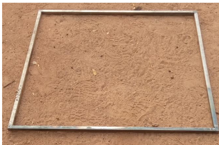
Fig. 3. Metallic device for observing biological crusts on the ground
